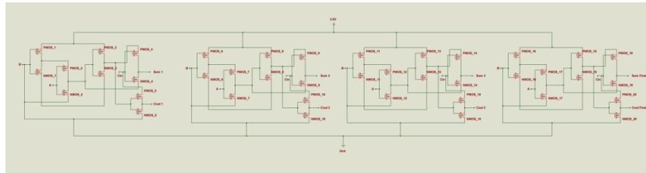
**Fig. 3** 4-Bit Full Adder using XNOR logic by GDI Technique
