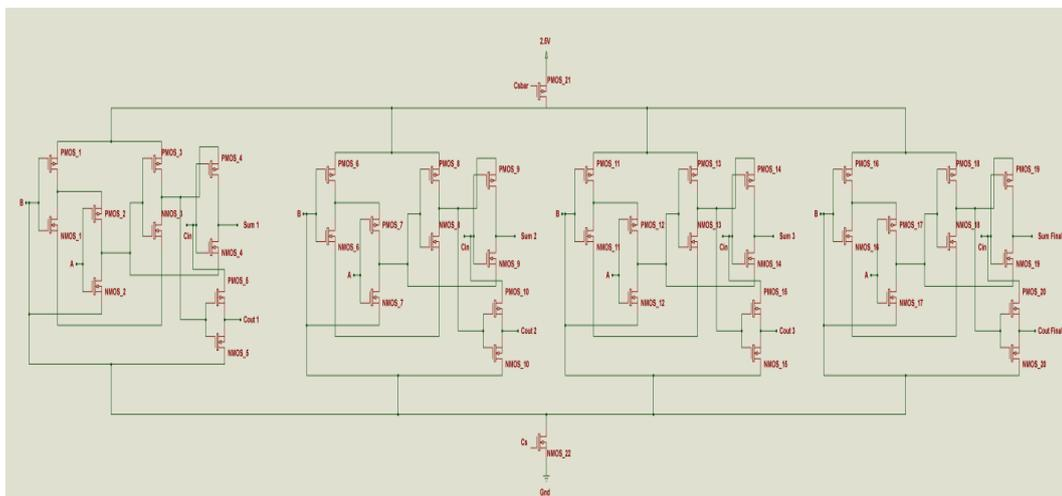
**Fig. 4** 4 bit XNOR based Full Adder using GDI technique with Header and Footer transistor (Proposed Design)
