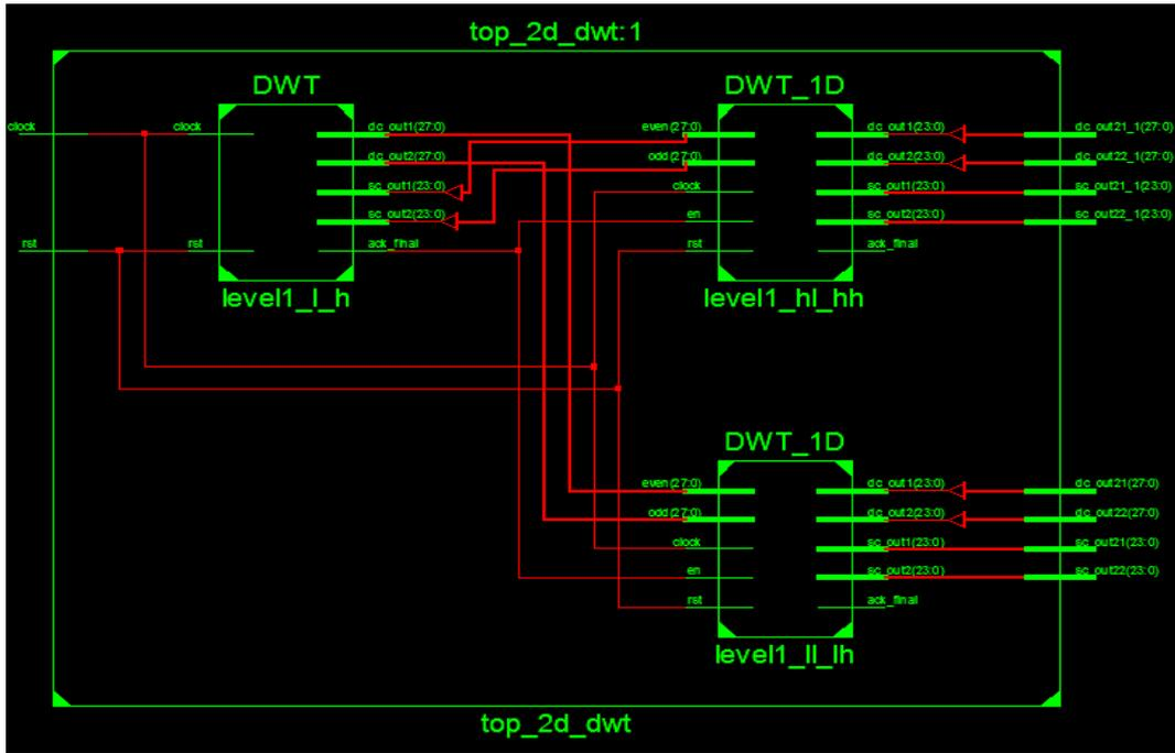
**Figure 9:** RTL schematic view of top 2D-DWT
