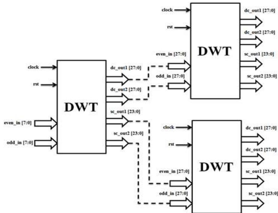
Figure 5: Architecture of 2D- DWT
