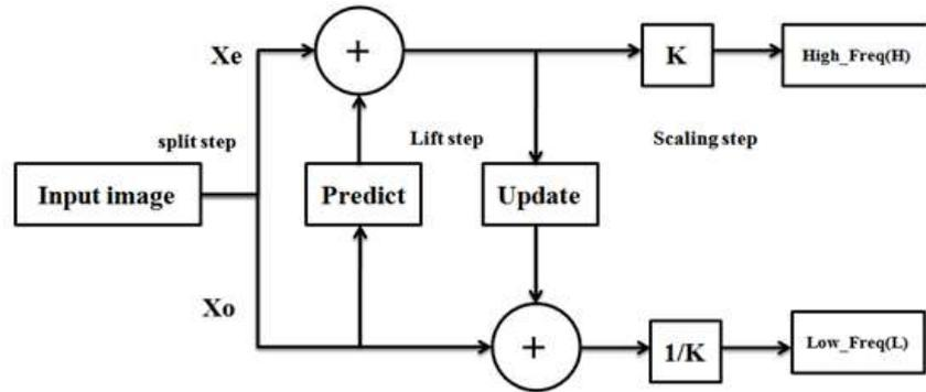
Figure 1: Forward Lifting Scheme using 5/3 wavelets transform
