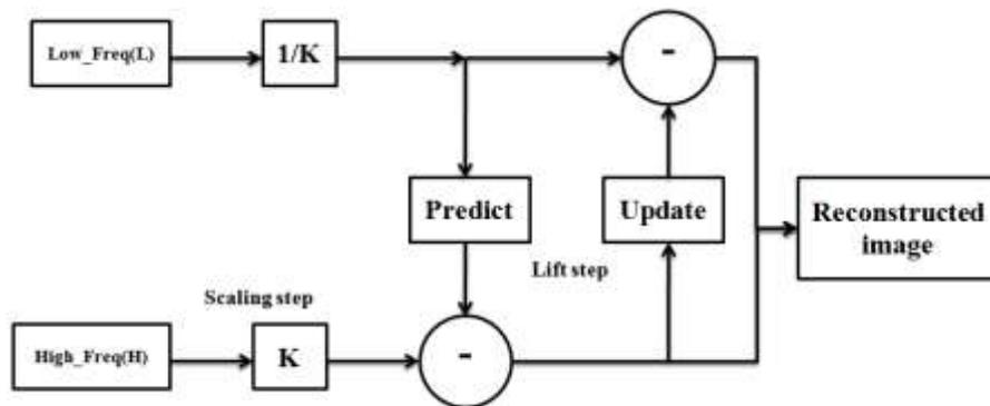
Figure 2: Backward Lifting Scheme using 5/3 wavelets transform
