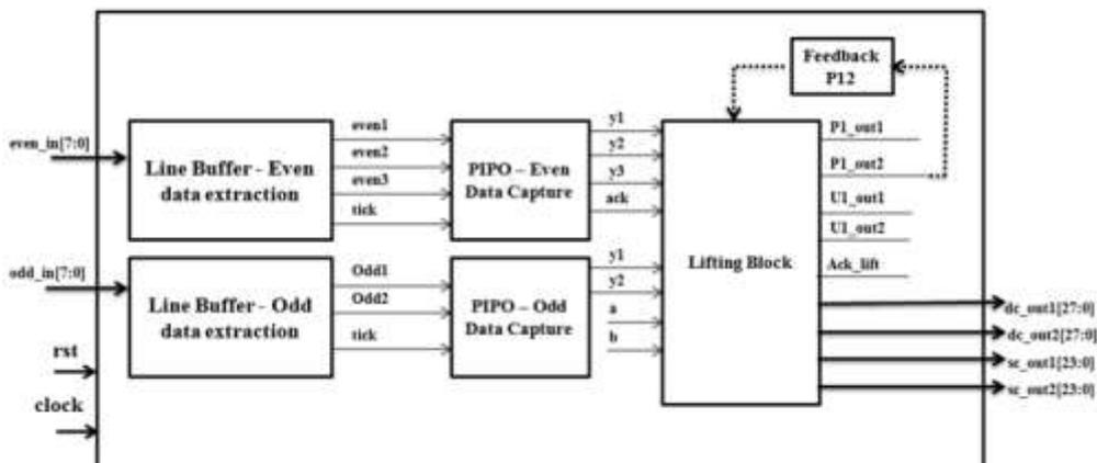
**Figure 4:** Building blocks of 1D-DWT
