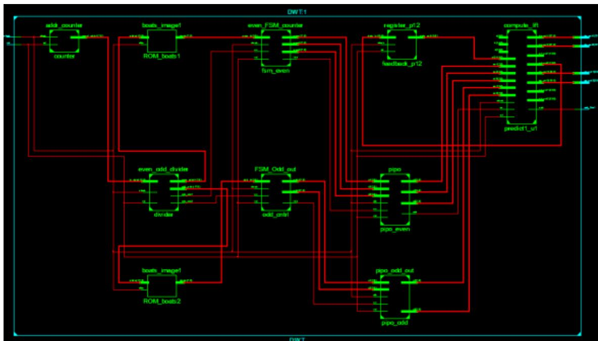
Figure 8: RTL Schematic View of Structured 1D-DWT
