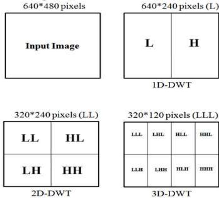
Figure 11: Image decomposition in 1D, 2D and 3D-DWT
