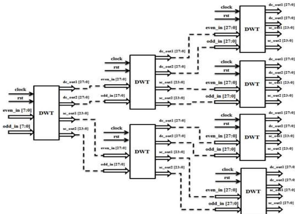
Figure 6: Architecture of 3D-DWT
