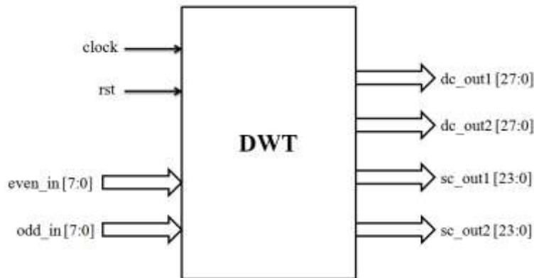
**Figure 3:** Top level architecture of 1D-DWT
