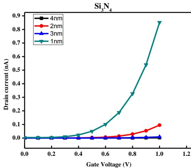
Figure 5 DG-FET transfer characteristics for 4 to 1 nm dielectric thickness variation
