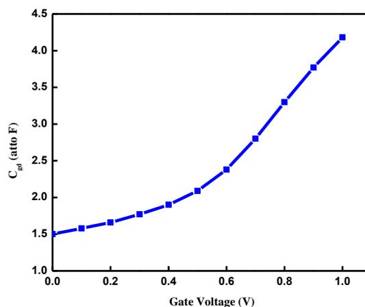
Figure 6 Gate-to-drain (C<sub>gd</sub>) capacitance at 4 nm dielectric thickness
