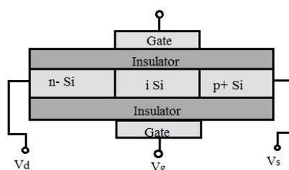
Figure 1 Basic Structure of Double-Gate FET [17]
