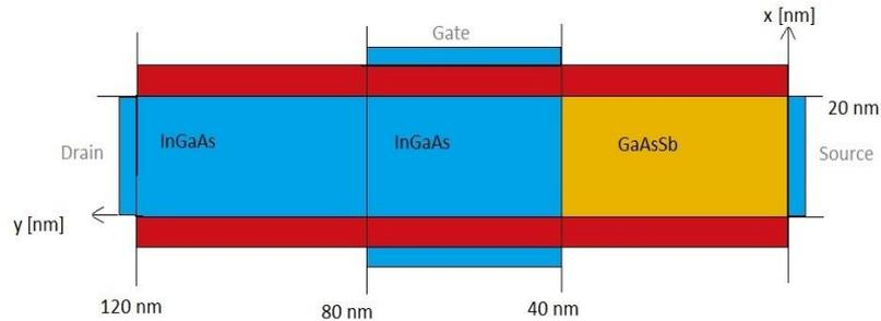
Figure 2 Structure of designed vertical DG-Tunnel FET
