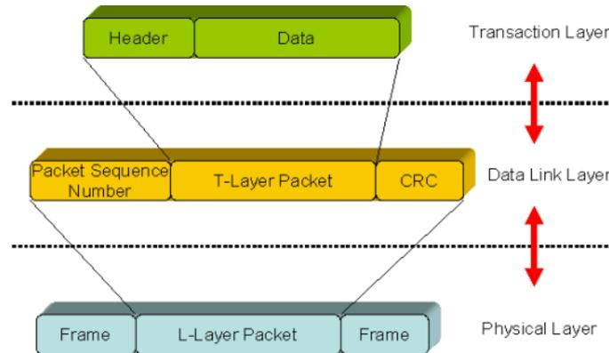
Figure 4: The data link layer adds data integrity features <sup>[1]</sup>.
