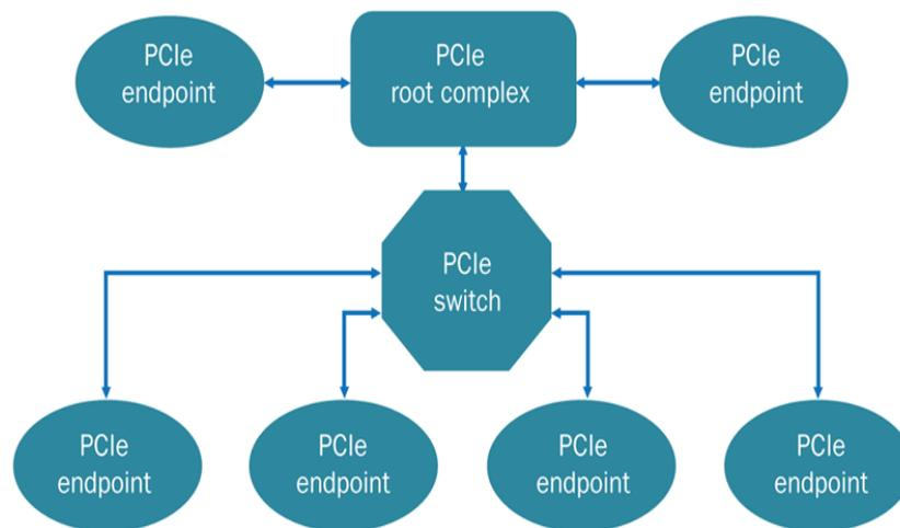
Figure 3: The PCIe Topology<sup>[8]</sup>.
