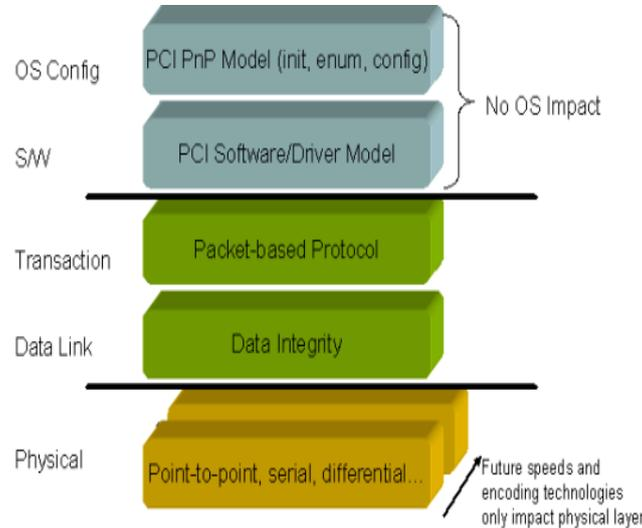
Figure 2: The PCI Express Architecture<sup>[1]</sup>.
