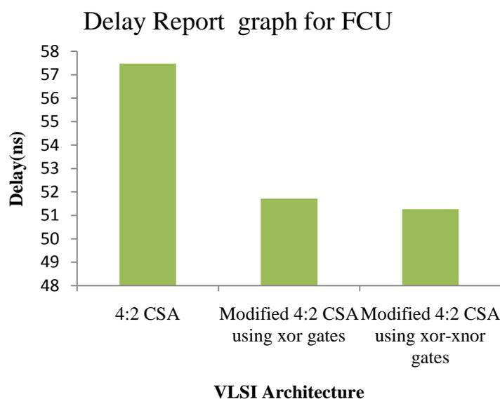
**Fig.20. Comparison of delay for VLSI architectures of FCU using different adders**
