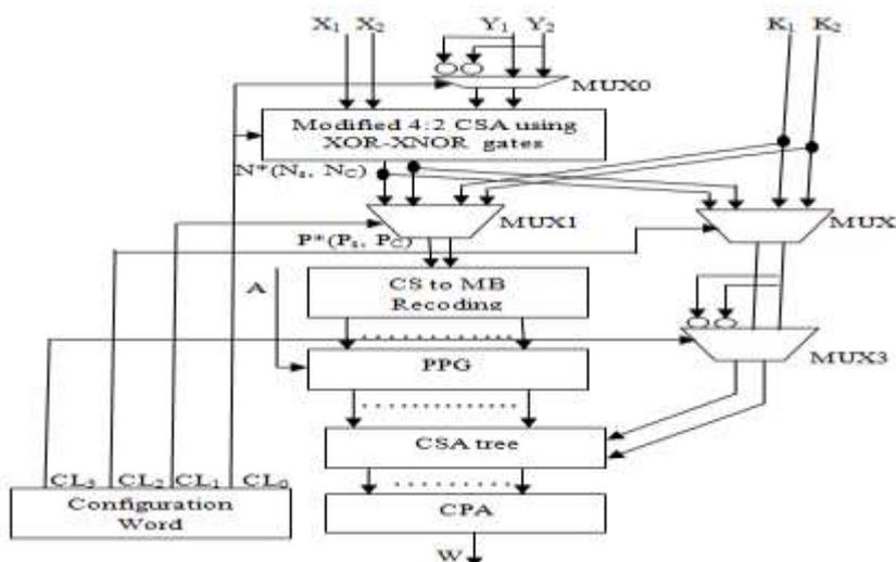
Fig.2. Block diagram of Flexible Computational Unit (FCU)
