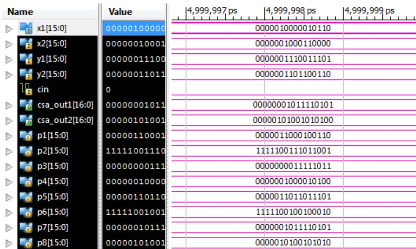
Fig.5. Simulation result of Modified 4:2 CSA using xor-xnor gates
