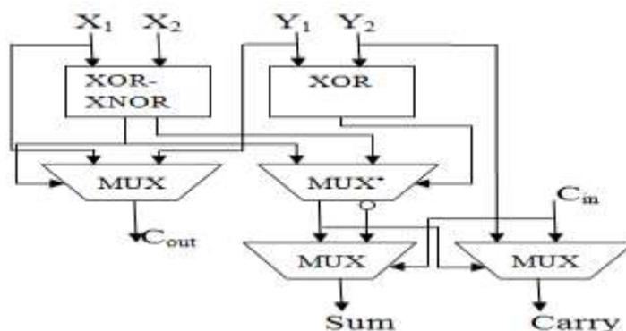
Fig.3. Modified Carry Save Adder using XOR- XNOR gates
