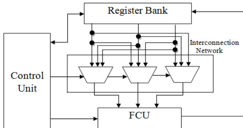
Fig.1. Block diagram of reconfigurable Flexible Data Path.
