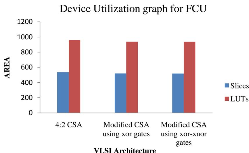
**Fig.19. Comparison of area for VLSI architectures of FCU using different adders**
