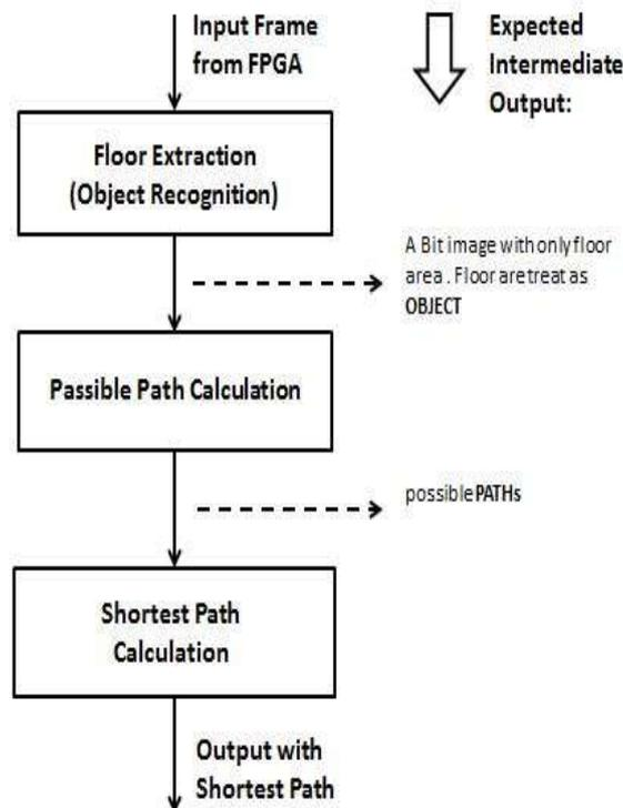
Fig.9. Flowchart of Path calculation algorithm
