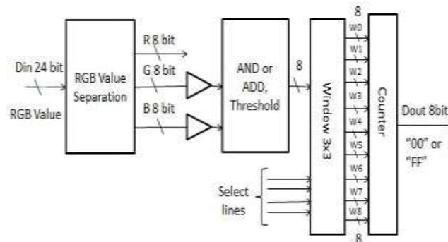
Fig. 5. Architecture of proposed FPGA module
