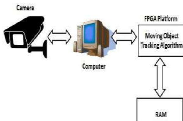
Fig.2: Layout of the Image Processing System
