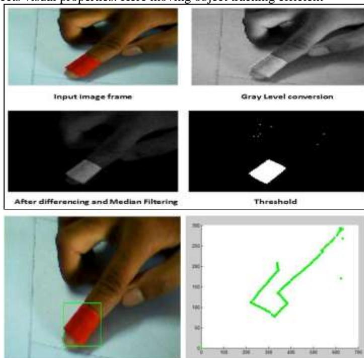
**Fig.12.** MATLAB simulation for moving object tracking
