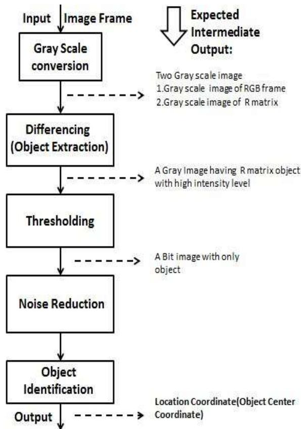
Fig.3: Algorithm Design for Object Recognition
