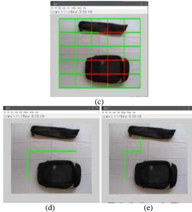
**Fig.11.** Path finding results (a) Original image (b) Floor extracted image (c) Possible movable paths shown in green (d) (e) shortest path output with two different destination coordinate
