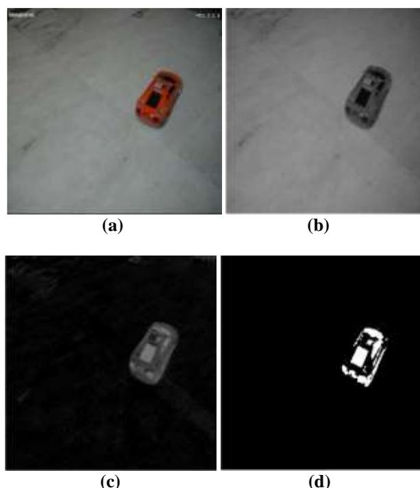
**Fig.4:** MATLAB simulation for moving object tracking (a) Original image (b) Gray image (c) after differencing (d) Thresholding.
