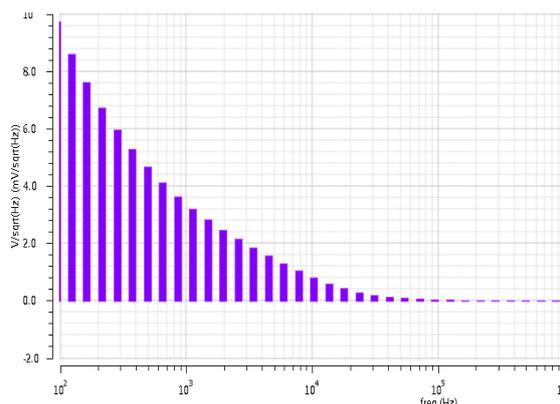
Fig. 7 Output Noise analysis of Two-Stage OP amp.
