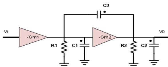
Fig. 1 Two-Stage MC amplifier structure.
