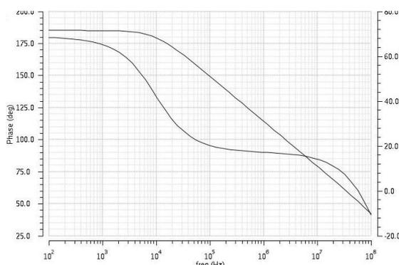
Fig. 6 Gain and Phase analysis of Two-Stage OP amp
