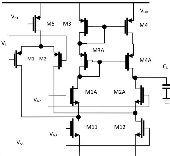
**Fig. 3** Folded-Cascode OP amp with PMOS input
