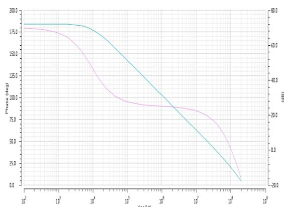
Fig. 8 Gain and Phase of Differential Folded-Cascode OP amp
