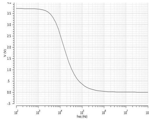
**Fig. 5** AC analysis of Two-Stage MC OP amp
