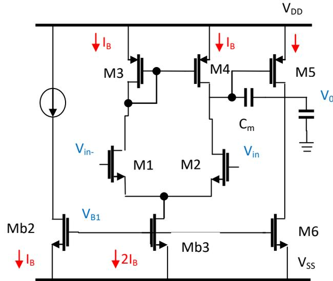
Fig. 2 Two-stage MC amplifier circuit structure.
