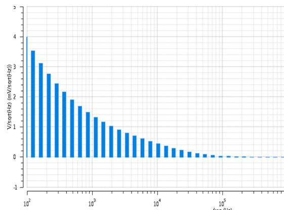
Fig. 9 Output Noise of Differential Folded-Cascode OP amp
