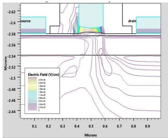
Fig.12 Electric field lines of Strained Si-pMOSFET
