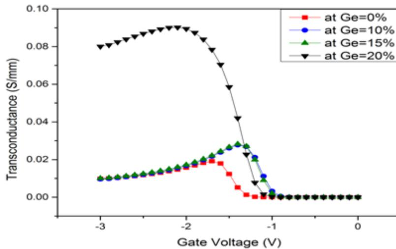
**Fig.8** Transconductance at different Ge Concentration
