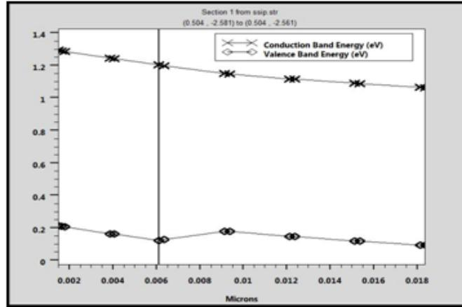
Fig.4 Energy band Structure at the interface of Strained Si and Si<sub>0.8</sub>Ge<sub>0.2</sub>
