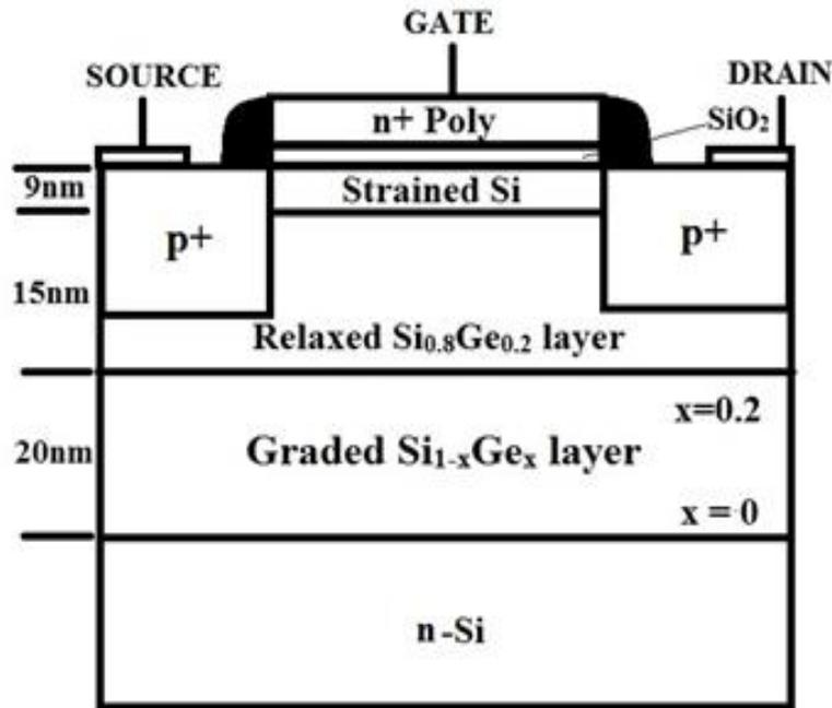
Fig.2 Cross Sectional View of Strained Si-pMOSFET
