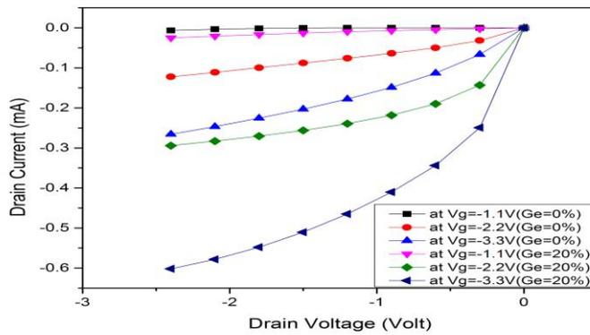
Fig.6 Output Characteristic ( $I_D \sim V_D$ ) Curve
