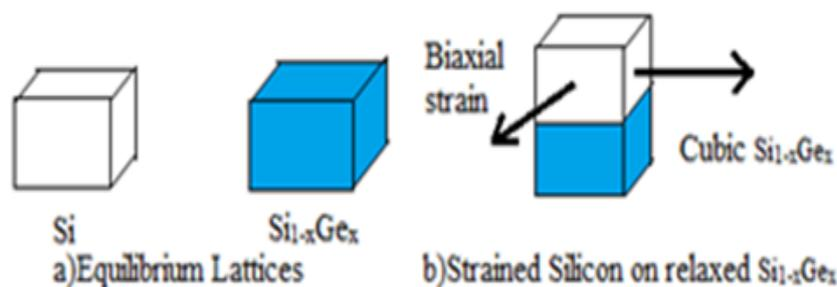
Fig.1. Schematic illustrations of (a) equilibrium lattices, (b) pseudomorphic strained Si on relaxed Si<sub>1-x</sub> Ge<sub>x</sub>.
