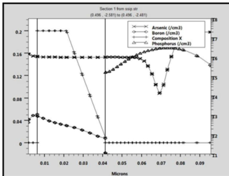
Fig.3 Concentration profile view of the 45nm St-Si pMOS
