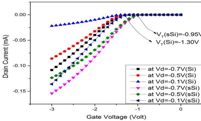
Fig.5 Current Drive Characteristic( $I_D \sim V_{GS}$ ) Curve
