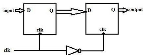
Fig.1 Master-slave flip-flop.
