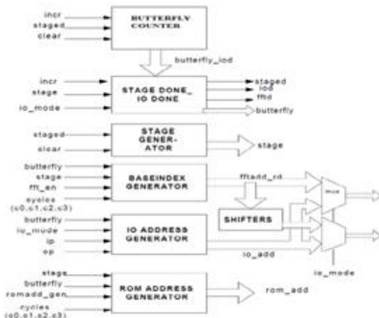
Figure 9: Architectural block diagram of Address Generation Unit.
