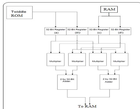
**Figure 33** Architecture of Twiddle Unit
