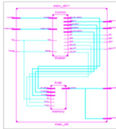
**Figure 39 :**RTL schematic of master control unit and RAM
