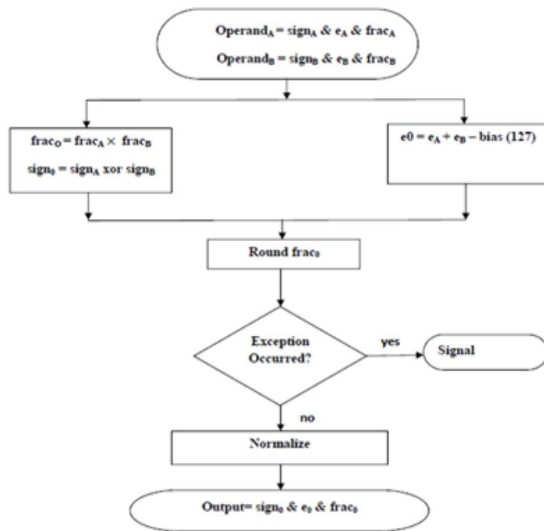
**Figure 36** Flowchart of floating point multiplier
