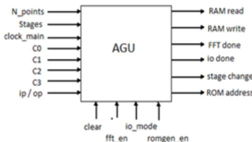
Figure 8. Block schematic of implemented AGU
