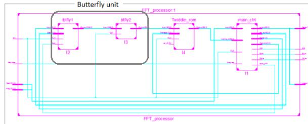
**Figure 43 :**RTL schematic of 1-D FFT using Radix-4 butterfly
