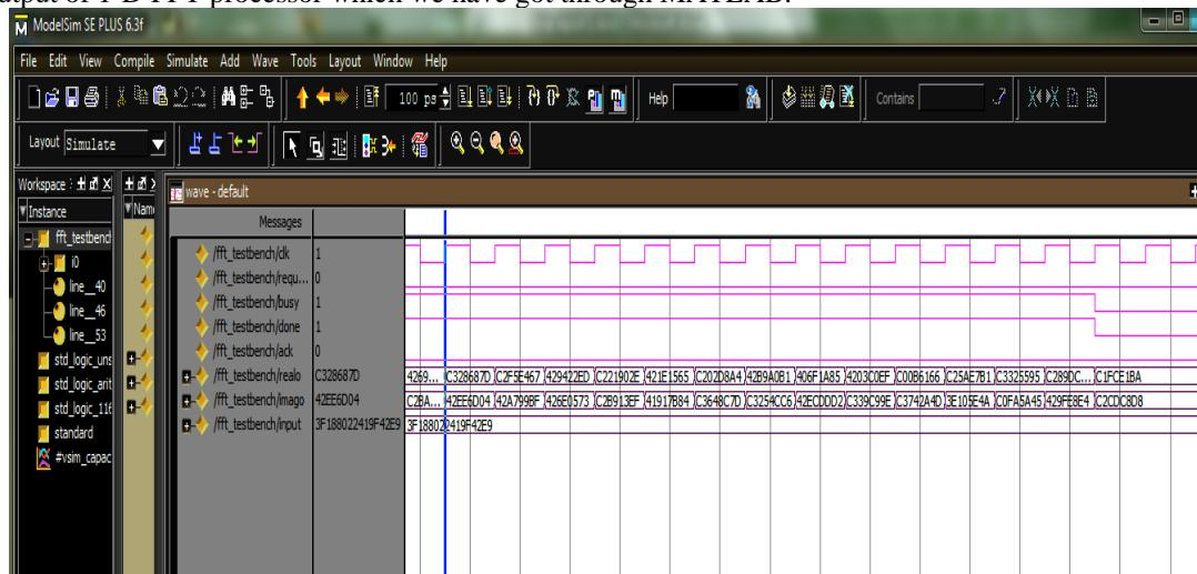
**Figure 46 :** Simulation Results of 16 point 1-D FFT using Radix-4
