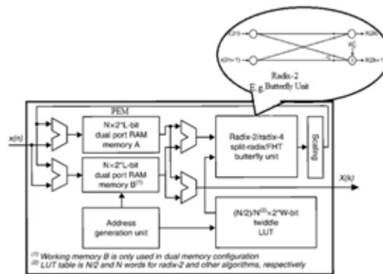
**Figure 3.** Block Diagram of 1-D FFT with single butterfly element
