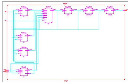
**Figure 40** RTL schematic of Butterfly element 1
