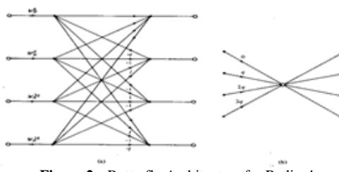
Figure 2. Butterfly Architecture for Radix-4
