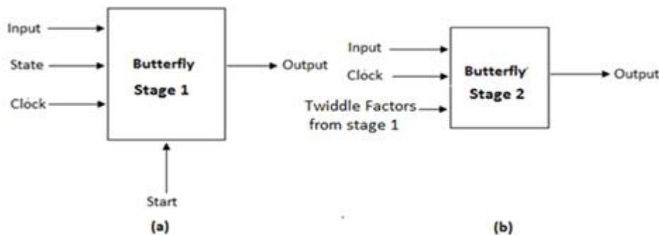
**Figure 32** Block schematic of Radix-4 Butterfly processing unit
