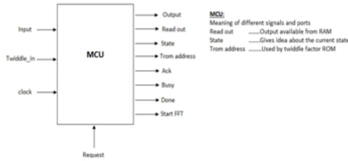
**Figure 28** Block schematic of implemented MCU
