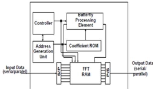
**Figure 5.** Architecture of 1-D FFT processor using Radix-2 Butterfly elemen
