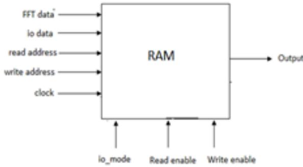
**Figure 14.** Block schematic of implemented RAM.
