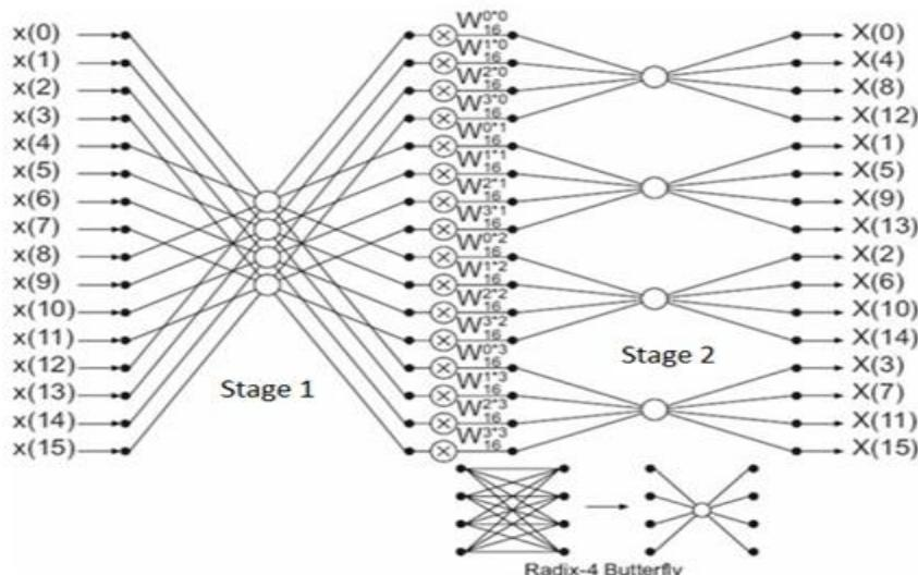
**Figure 26** Signal flow graph of 16 point Radix-4 FFT
