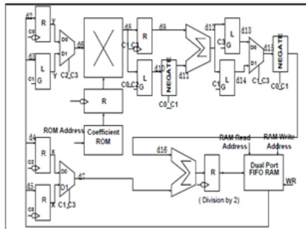
**Figure 12.** Radix-2 Butterfly Processor
