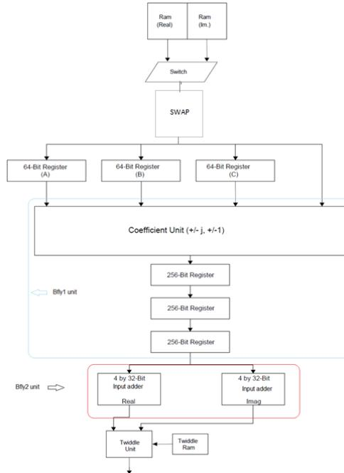
**Figure 30** Radix-4 Butterfly processing unit
