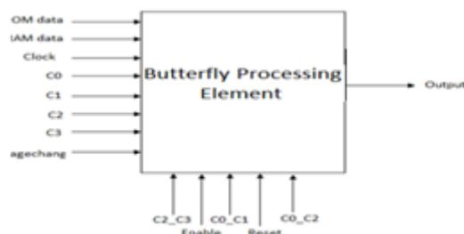
**Figure 11.** Block schematic of Butterfly PE
