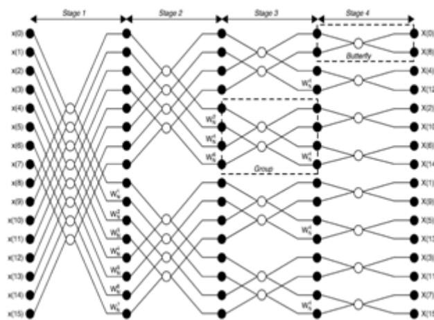
**Figure 4.** signal flow graph of 16 point DIT FFT
