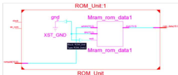
**Figure 20** RTL schematic of ROM
