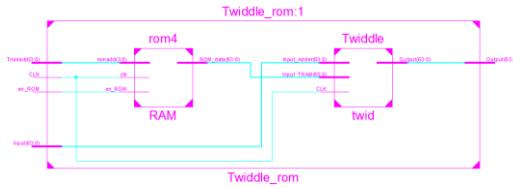
**Figure 42:**RTL schematic of twiddle ROM
