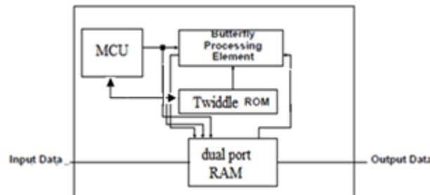
Figure 25 Architecture of 1-D FFT using Radix-4 butterfly element
