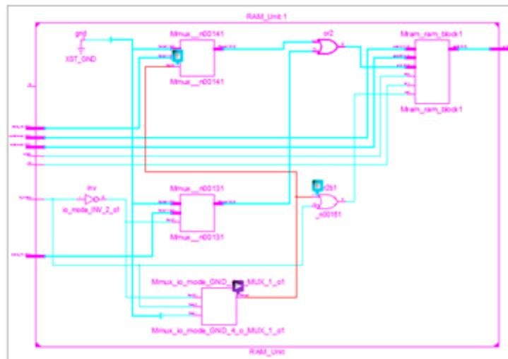
**Figure 19** RTL schematic of RAM.
