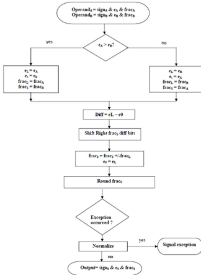
**Figure 37** Flowchart of floating point adder
