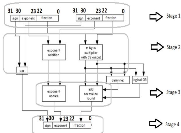
**Figure 35** Floating point Multiplier
