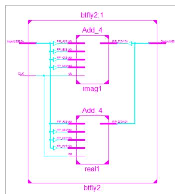
**Figure 41** ;RTL schematic of butterfly element II
