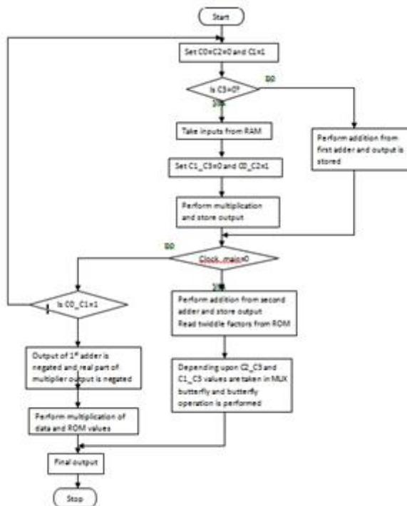
**Figure 13.** Flow chart of Butterfly processing element.
