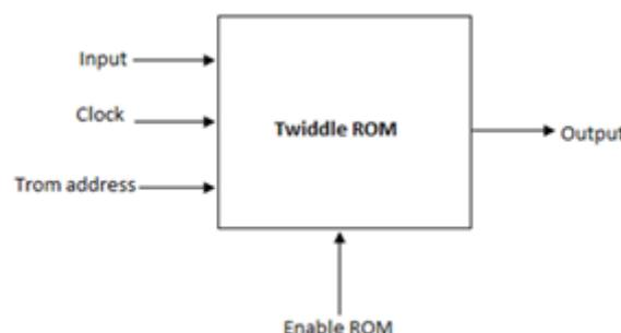
**Figure 34** Block schematic of implemented twiddle ROM
