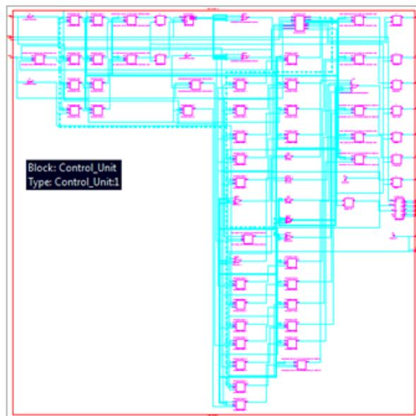
**Figure 16.** RTL schematic of Master Control Unit.
