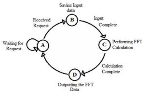
**Figure 27** State diagram of MCU
