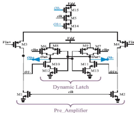
Fig. 4. Low-power two stage dynamic comparator
