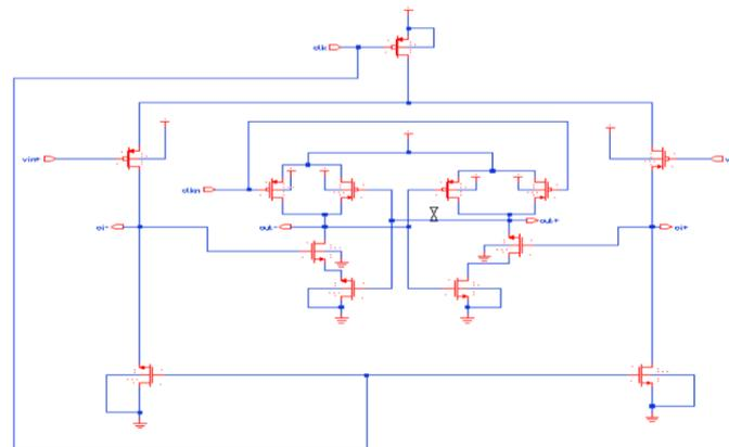
**Fig. 2** Two stage dynamic comparator schematic diagram
