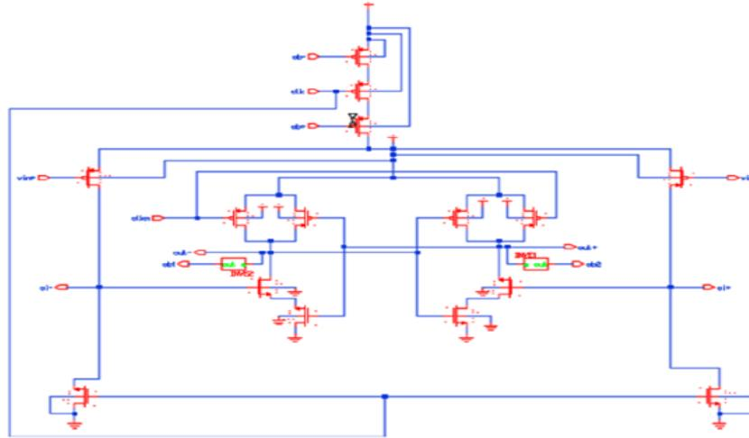
Fig.5 Low –power two stage dynamic comparator schematic diagram
