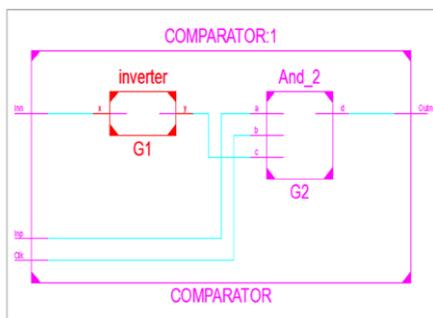
Fig 12.Internal RTL schematic 1
