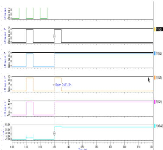
Fig.14. Waveforms of Conditional Evaluated Domino Logic
