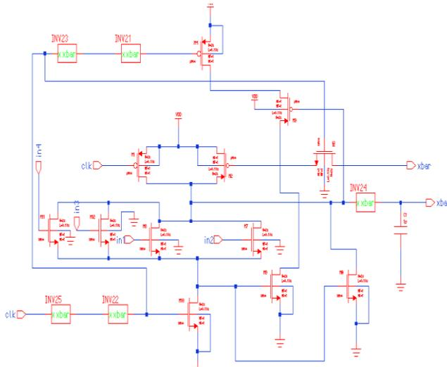
Fig. 15 Conditional Stacked Keeper Domino Logic
