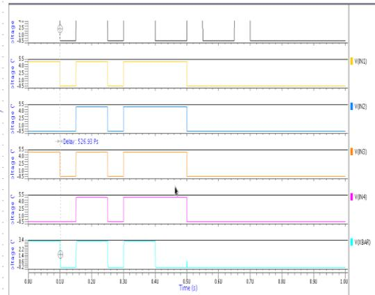
Fig 5. Waveforms of Footed Domino Logic
