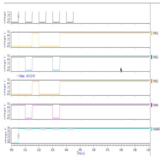
Fig. 12. Waveforms of Modified High Speed Clocked Delay Domino Logic
