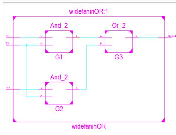
**Fig 21.**RTL schematic
