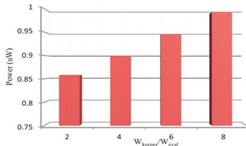
**Fig.3** Effect of keeper sizing on power consumption of FLDL domino logic circuit
